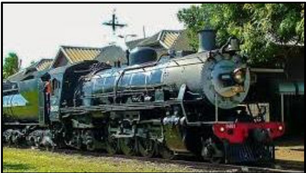
Under the Whyte notation system, a steam locomotive that has two leading wheels arranged in a leading truck, eight coupled driving wheels and four trailing wheels in a trailing truck is designated a 2-8-4.
