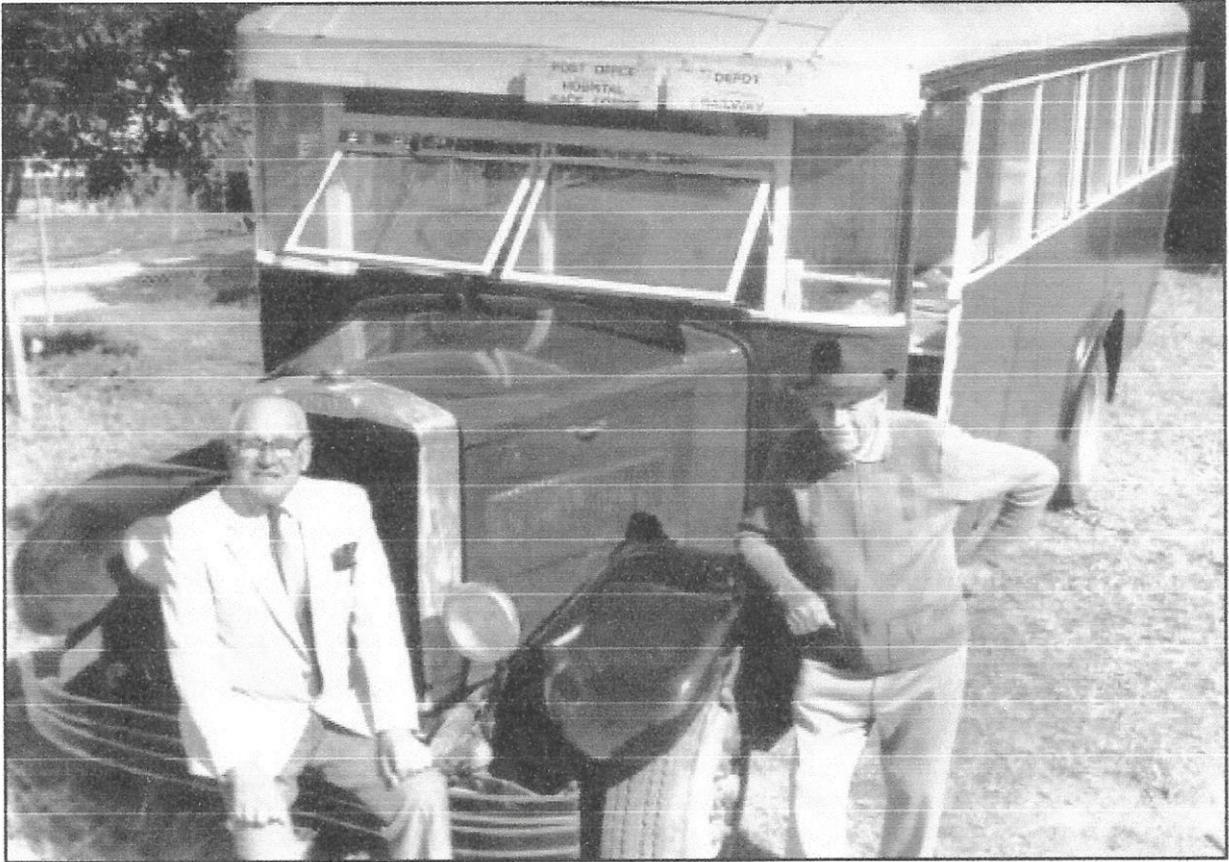
The late Reg Lewis and his brother Clarrie are pictured here with their 1932 Leyland Cub KP3 151 omnibus, which operated on the Red Hill-Stewart Terrace run. It is powered by a 4.4 litre, 27 horsepower petrol engine, and was licenced to carry 22 passengers. It was purchased (along with a Bedford bus) in 1932 after Clarrie won the lottery. During the second World War it was run on kerosene, or producer gas from a charcoal burner. The Lewis brothers operated the bus service until 1975.
